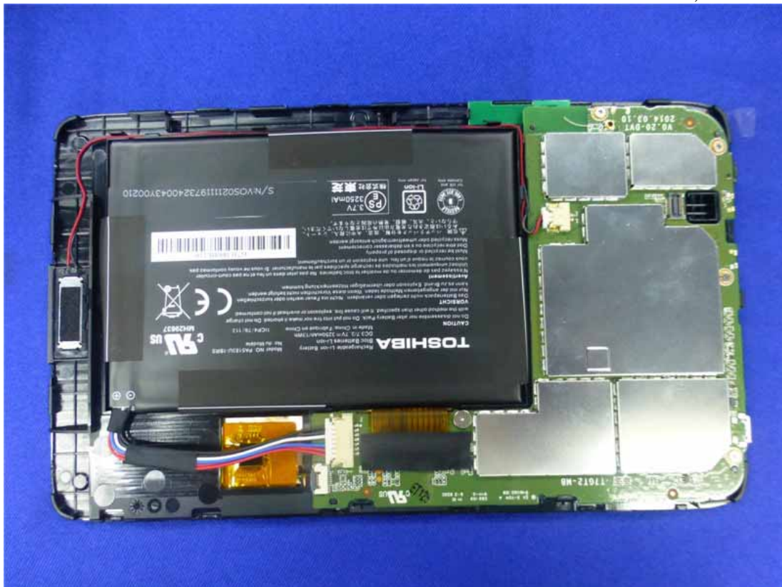
Figure 16 Without Rear Camera, Inside of the EUT
