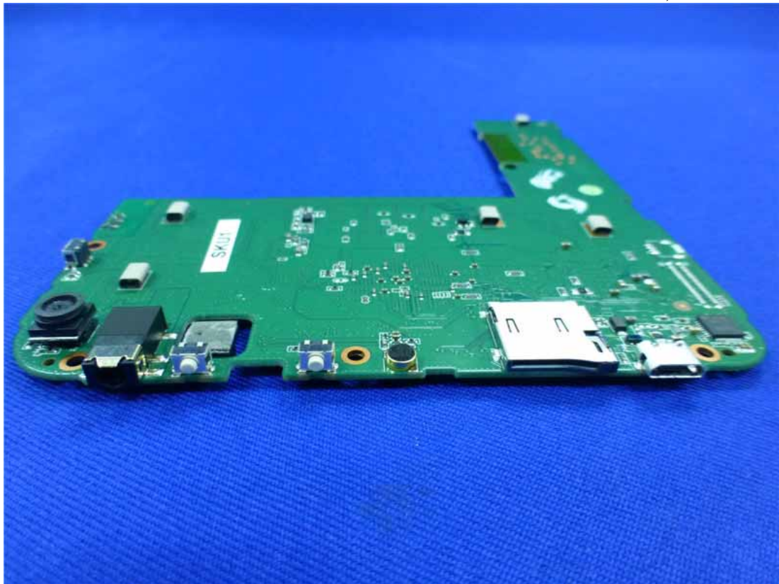
Figure 10 With Rear Camera, I/O Port of the PCB
