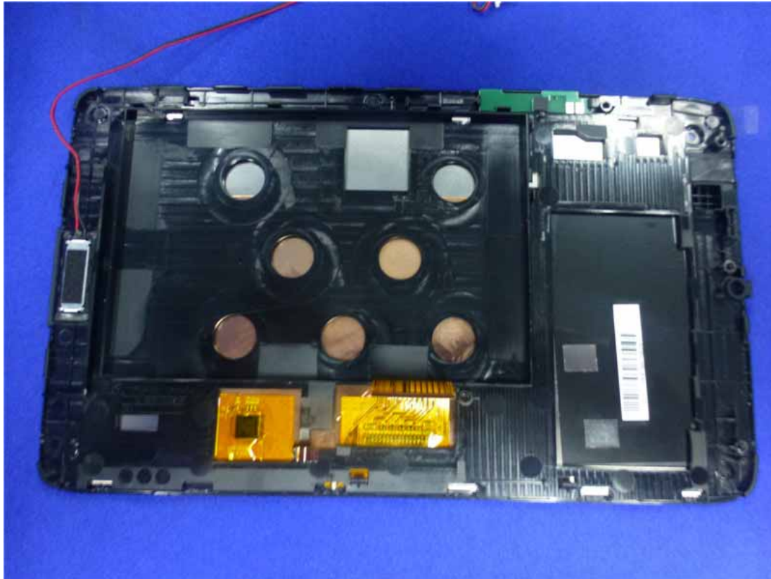
Figure 21 Backside of the LCD Panel
