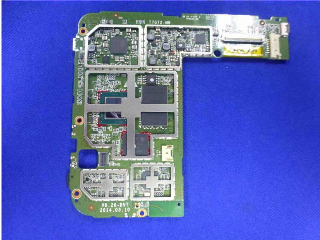
Figure 17 Without Rear Camera, Component side of the PCB
