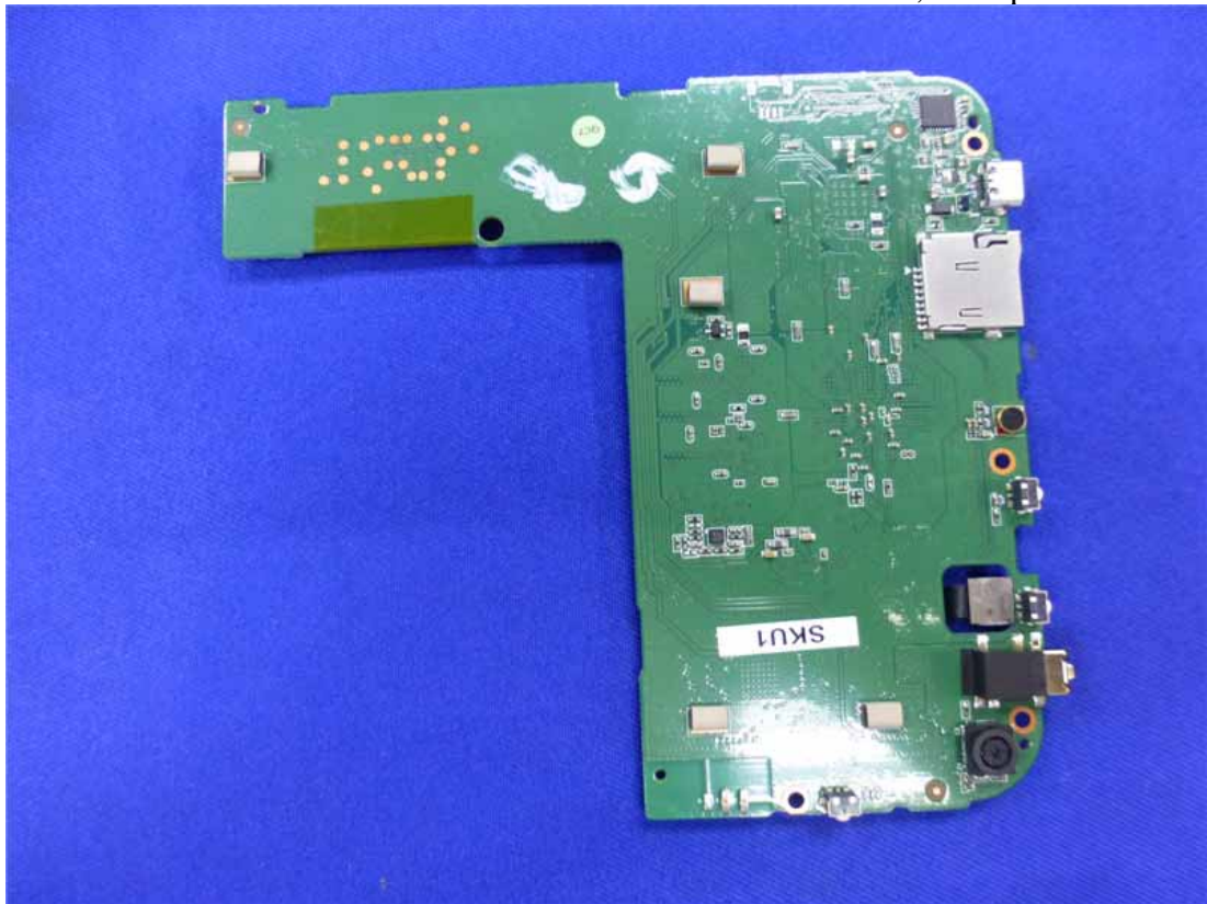
Figure 9 With Rear Camera, Component side of the PCB
