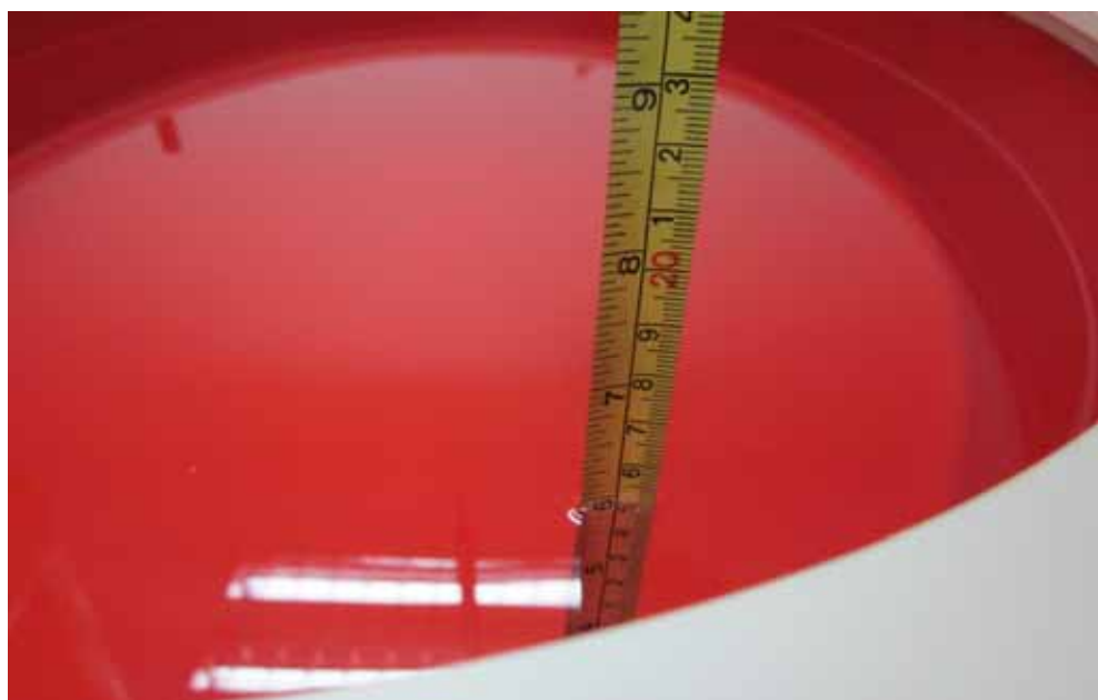
Figure 4.4: Liquid depth in the Flat Phantom
