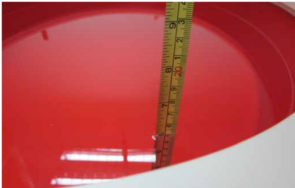
Figure 4.4: Liquid depth in the Flat Phantom
