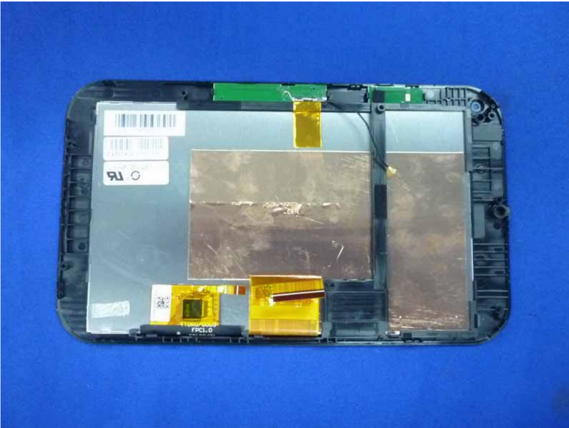
Figure 10 Backside of the LCD Panel
