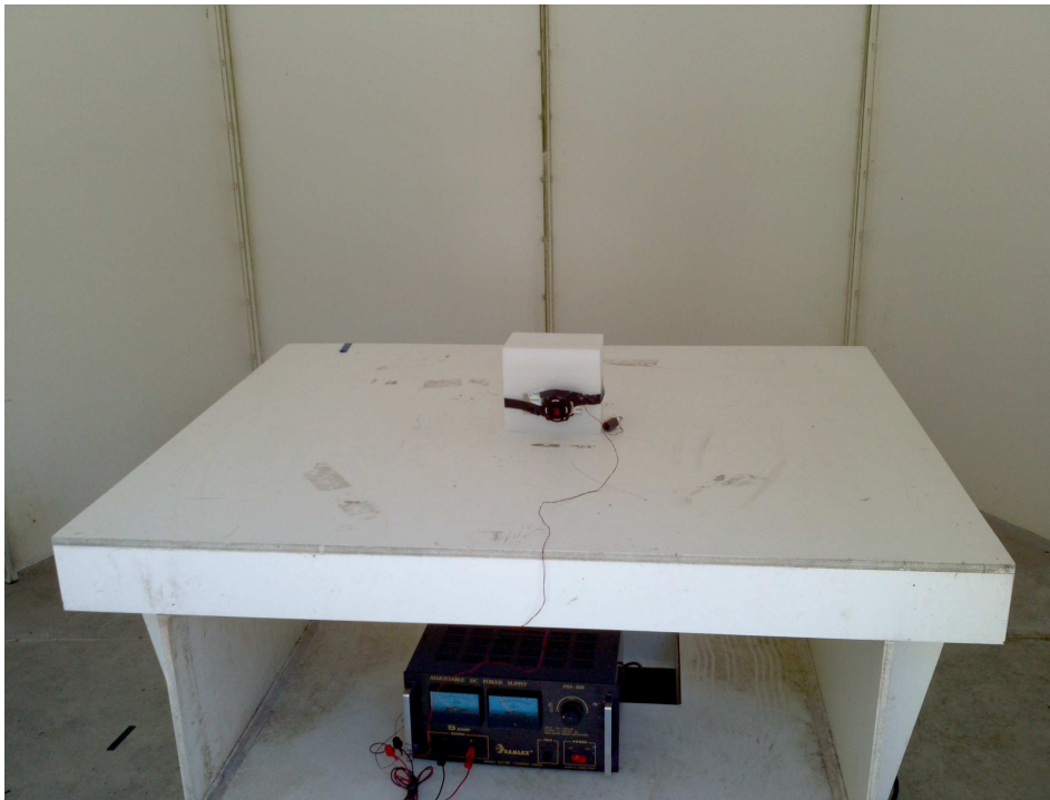
Picture 2: Radiated Emissions Test Setup at Open Area Test Site
