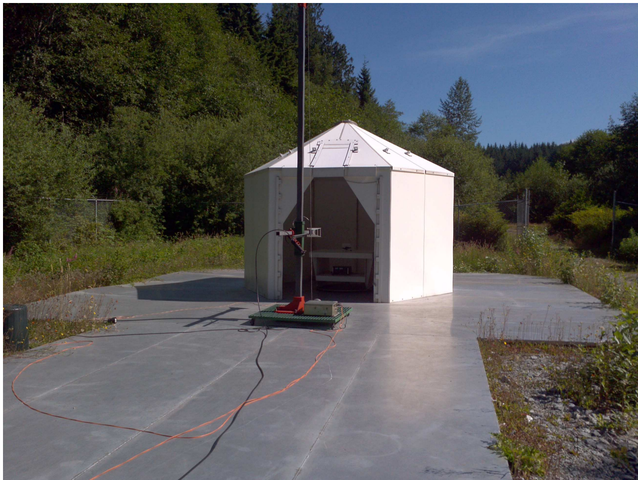
Picture 3: Radiated Emissions Test Setup at Open Area Test Site
