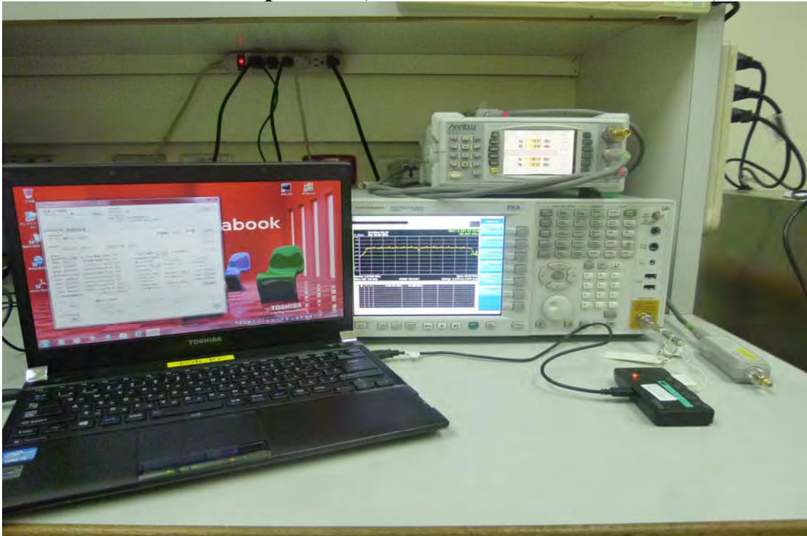
Conducted Setup Photo (Measurement at Antenna Port)
