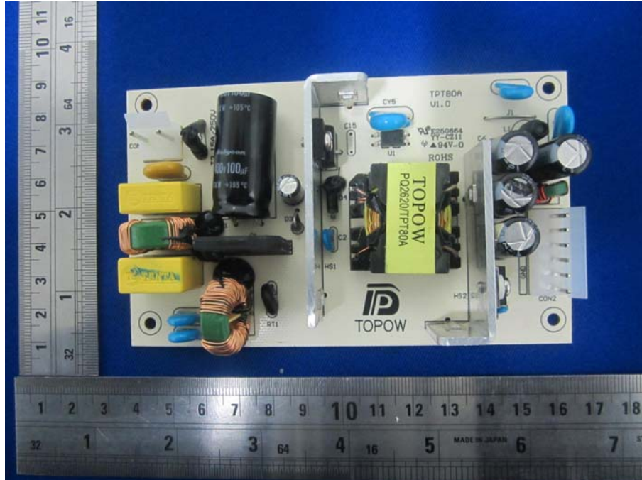
EUT – Power Supply Top View
