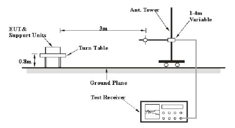
The radiated emission tests were performed in the 3 meters chamber test site, using the setup accordance with the ANSI C63.4-2009. The specification used was the FCC Part 15.109, Class B limits.
