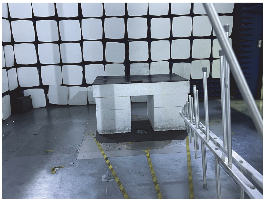
Radiation Emission Test Setup (30MHz to1GHz)
