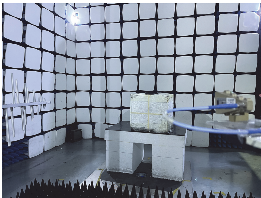
Radiation Emission Test Setup (Above18GHz)
