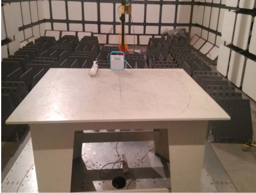
Radiated Emissions – Front View (1-25 GHz)
