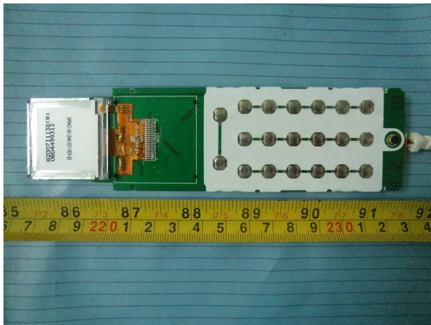
EUT – Main Board Bottom LCD off View (Handset)
