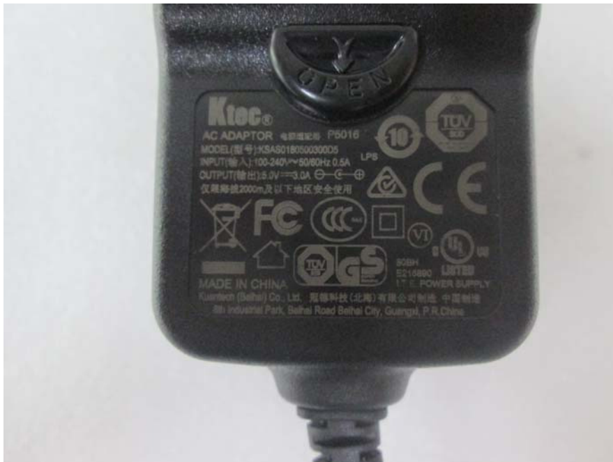
EUT –Adapter Label View
