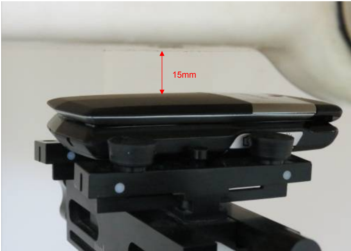
Picture 13: Body, The EUT display towards phantom, the distance from EUT to the bottom of the Phantom is 15mm (Closed)
