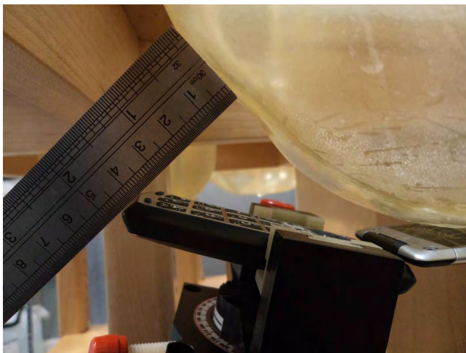
Left Head Touch Setup Photo (The distance between SAM and EUT antenna location is 4.5cm)
