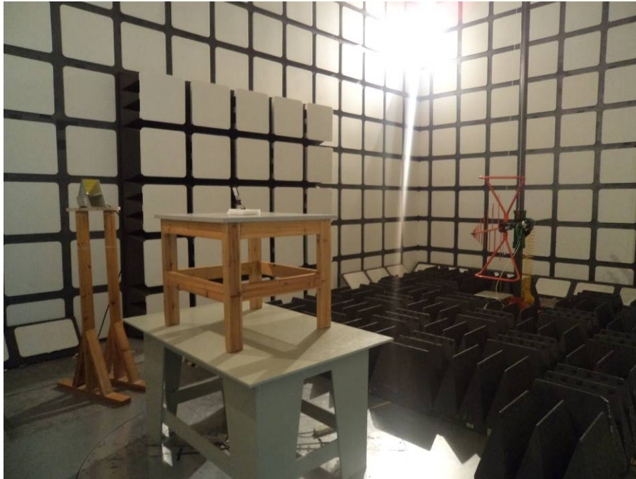
Below 1GHz: Radiated Emissions - Front View
