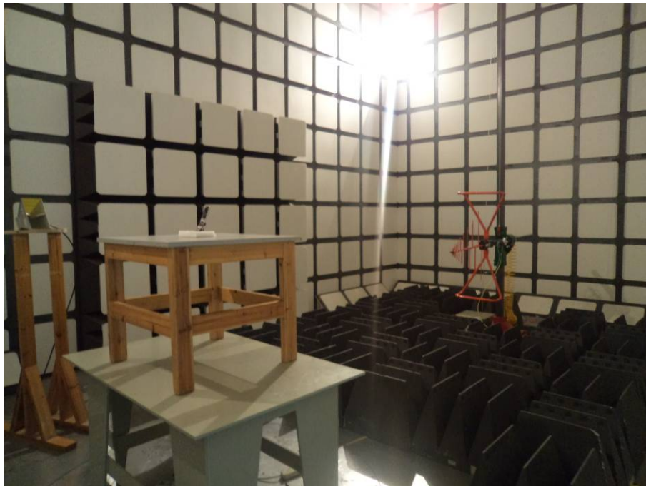
Below 1GHz: Radiated Emissions - Rear View
