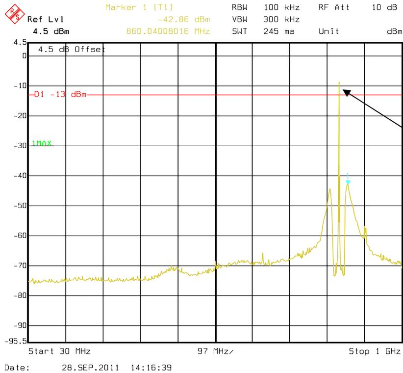
Fundamental test with Band Reject Filter
