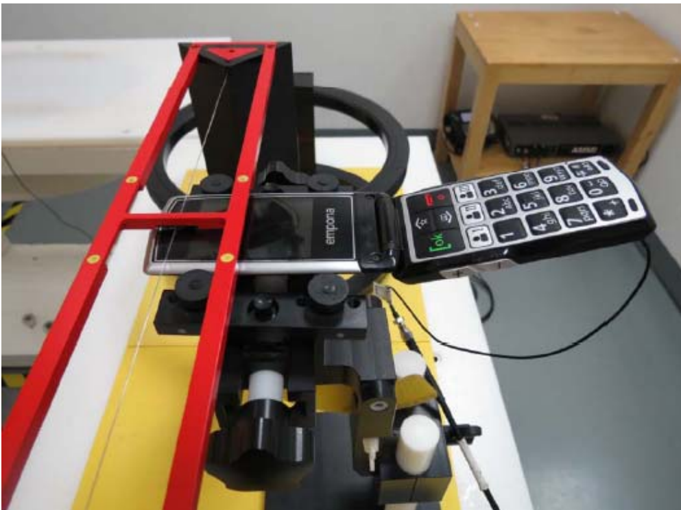
Photo 2: HAC T-Coil Set-up
