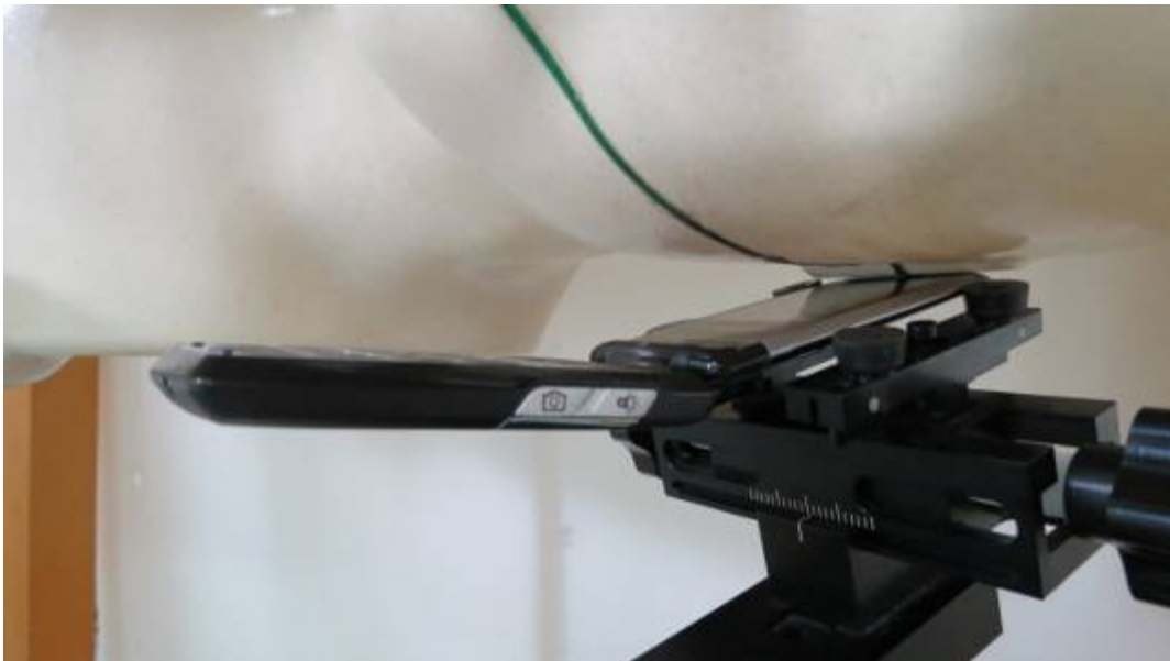
Picture 8: Left Hand Tilt 15 Degree Position
