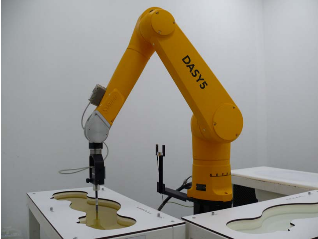
Picture 1: Specific Absorption Rate Test Layout
