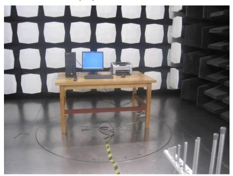
8. Part 15B Radiated emission(USB) above 1 GHz
