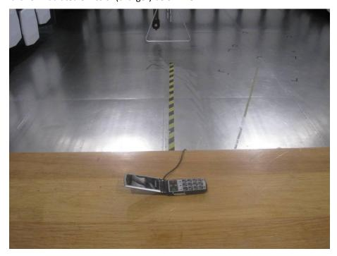
6. Part 15B Radiated emission(charger) Above 1 GHz
