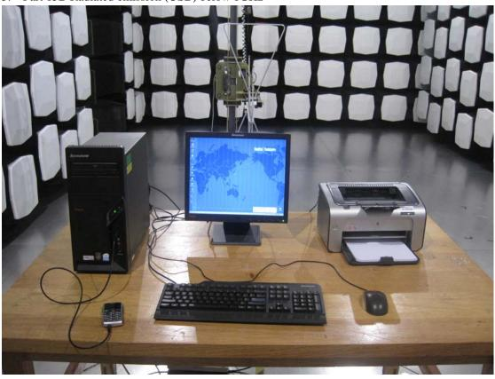
6. Part 15B Radiated emission (USB) above 1GHz
