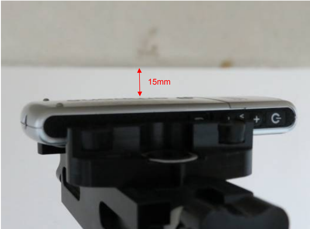
Picture 11: Body, The EUT display towards ground, the distance from EUT to the bottom of the Phantom is 15mm
