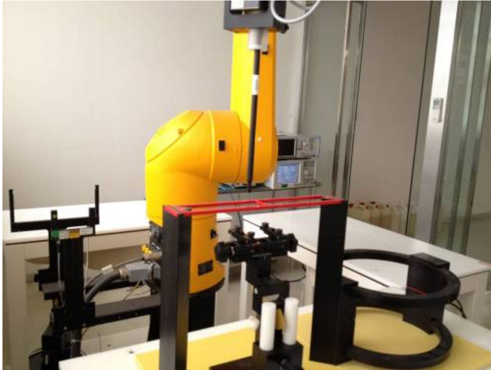
Picture A1: HAC RF System Layout
