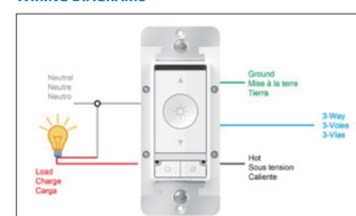
Single location control installation
