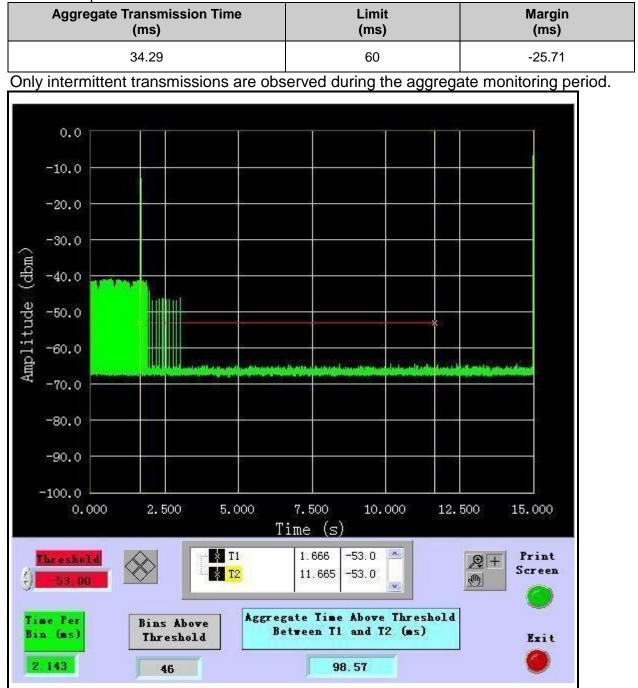
NOTE: Type 0 Radar signal trigger at T1, channel stop data transmission and move.
