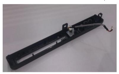
3. Fixed the front case subassembly to the bottom case subassembly
