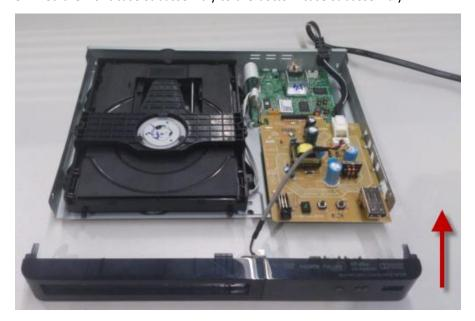
4. connected the WIFI cable to the mainboard 4-pins connector.
