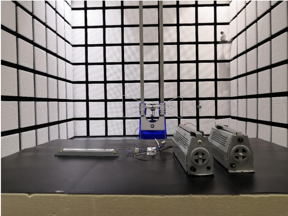
Radiated Emission test below 1GHz
