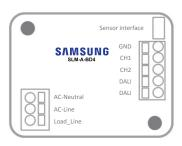
. Load Line should be connected with driver's AC input
