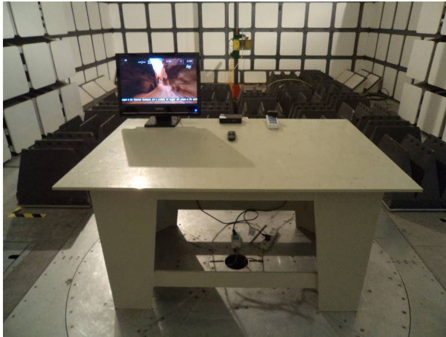
Radiated Emission - Front View (Above 1 GHz)
