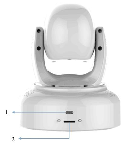
**1 Power Input Socket:** Connect Power adaptor, the adaptor's output is 5V 1.5A.
