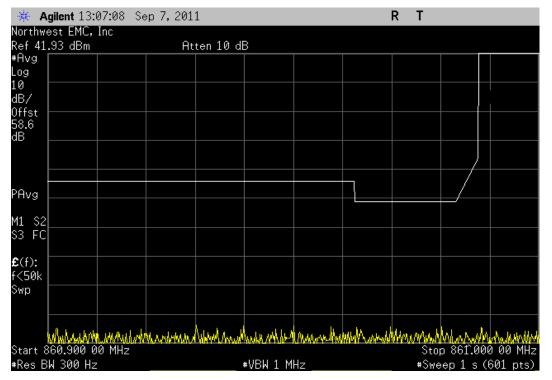
EVDO, Antenna Port A, Multi Carrier [5 FA], (862.9 MHz, 864.16 MHz, 865.4 MHz, 866.65 MHz, 867.9 MHz), Lower Band Edge Zoomed Out
