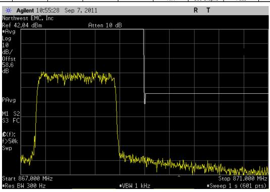
CDMA, Antenna Port B, Multi Carrier [5 FA], (862.9 MHz, 864.16 MHz, 865.4 MHz, 866.65 MHz, 867.9 MHz), Lower Band Edge Zoomed In
