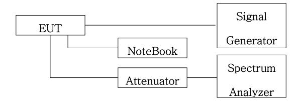
**Block Diagram 1. RF Power Output Test Setup**
