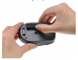
2. Install two AAA Batteries into your Mouse, replace the Battery Compartment Cover back onto your Mouse until it securely locks.
