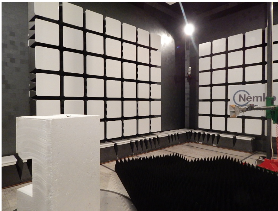
Figure 1-2: Emissions setup photo – above 1 GHz
