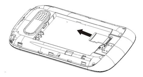
Aim at the memory card slot and push the memory card gently, and the card should be inserted correctly.
