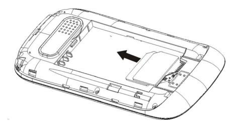
Metal contact surface of SIM card is easily scratched. You must take out SIM care carefully before the assembly.
