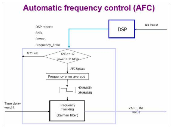
In MT6223, it uses a AFC signal from baseband (DAC) to finish automatic frequency control.
