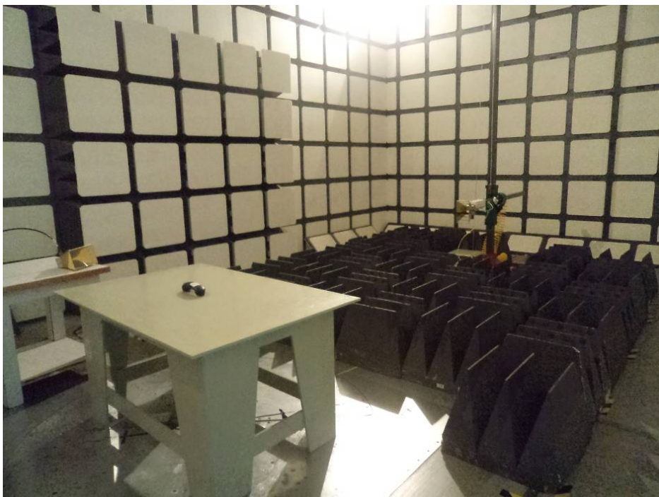
Radiated Emissions - Rear View (Above 1 GHz)
