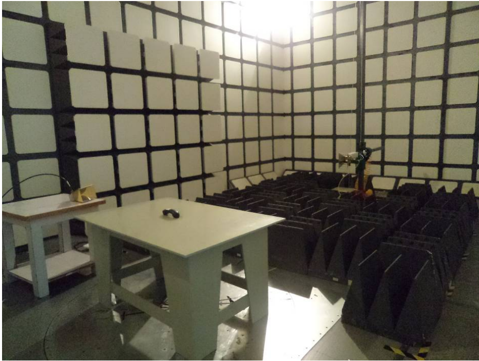
Radiated Emissions - Rear View (Above 1 GHz)
