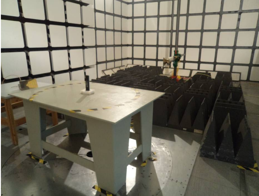
Radiated Emissions View
