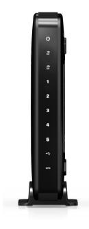
Power: Indicates when the Range Extender is powered on. The LED will remain on.
