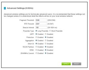
system to recover quicker from interference/collisions. Higher values provide the fastest throughput.
