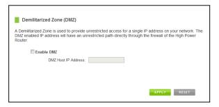
As a general safety rule, devices placed on the DMZ should not have any other network connections to any other devices.
