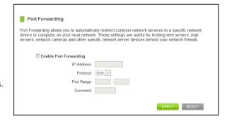
IP Address: The IP address of the device behind the Firewall that is being designated for Port Forwarding.
