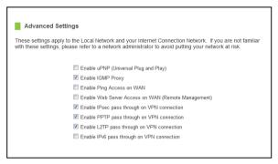
media, such as an Ethernet connection or wireless connection. With UPnP enabled, network devices may change security settings within the Router's firewall to allow access over the Internet. By default, UPnP is disabled to avoid exposing your network to security issues.
