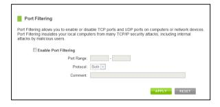
Hackers may sometimes scan for all open ports on your network as a method of hacking into your network. Port Filtering and other firewall features help to prevent this from happening.
