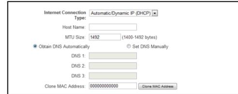
The screenshot shows a configuration window for Internet Connection Type. The 'Internet Connection Type' dropdown menu is set to 'Automatic/Dynamic IP (DHCP)'. Below this, there are fields for 'Host Name', 'MTU Size' (set to 1492), and three 'DNS' fields (DNS 1, DNS 2, DNS 3). There are two radio buttons: 'Obtain DNS Automatically' (selected) and 'Set DNS Manually'. At the bottom, there is a 'Clone MAC Address' field with the value '000000000000' and a 'Clone MAC Address' button.
