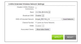
Broadcast SSID: Selecting Disable Broadcast SSID will hide the visibility of the Range Extender's SSID. Users must manually enter the SSID to connect.
