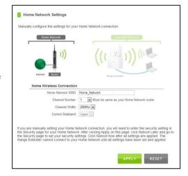
40Hz is 5-11. 40Hz allows for faster speeds. Select the channel width you wish to use for your network. This setting must match that of your Home Network for a successful connection.
