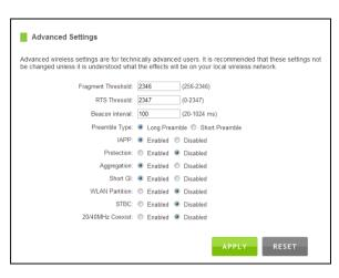
Preamble Type: Defines the length of the Cyclic Redundancy Check for communication between the Range Extender and roaming Wi-Fi users.
