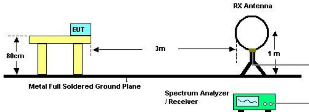
For Radiated Emissions: 30MHz~1GHz
