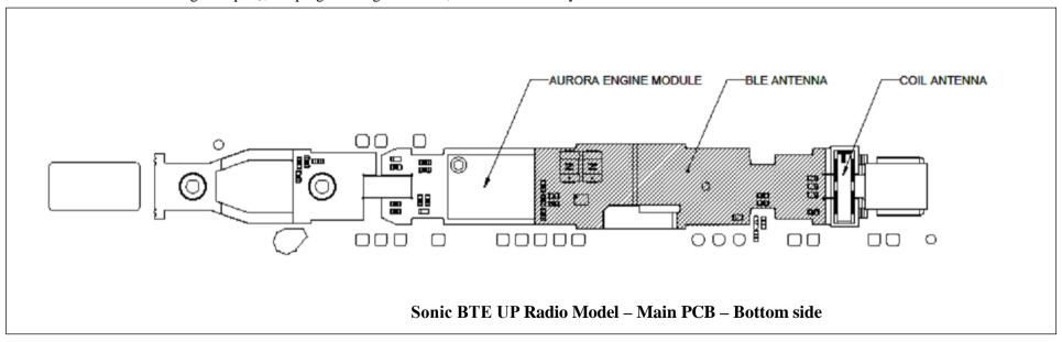
The most important parts inside the Engine module are a Digital-Signal-Processor (DSP), a radio Front-End (FE) chip for the 3.84 MHz radio part and an RF chip for the Bluetooth radio part – all mounted on a small rigid PCB again mounted on the main flex PCB. The Sonic BTE UP radio model also includes all voltage regulators and buffered data programming inputs on board. The DSP is the main processor controlling the functionality of both radios in the Sonic BTE UP radio model.
