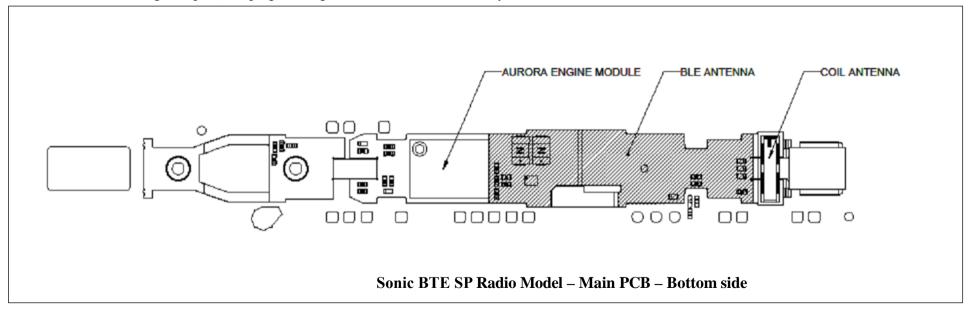
The most important parts inside the Engine module are a Digital-Signal-Processor (DSP), a radio Front-End (FE) chip for the 3.84 MHz radio part and an RF chip for the Bluetooth radio part – all mounted on a small rigid PCB again mounted on the main flex PCB. The Sonic BTE SP radio model also includes all voltage regulators and buffered data programming inputs on board. The DSP is the main processor controlling the functionality of both radios in the Sonic BTE SP radio model.
