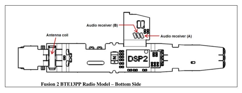
On the bottom side of the radio model the DSP, the antenna coil and pads for connecting the audio receiver can be seen.
