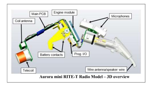
The radio model is implemented in an engine module mounted on the main PCB with connections to the antennas, the microphones, the speaker and the battery terminals. The radio model can be seen in 3D overview to the left:
