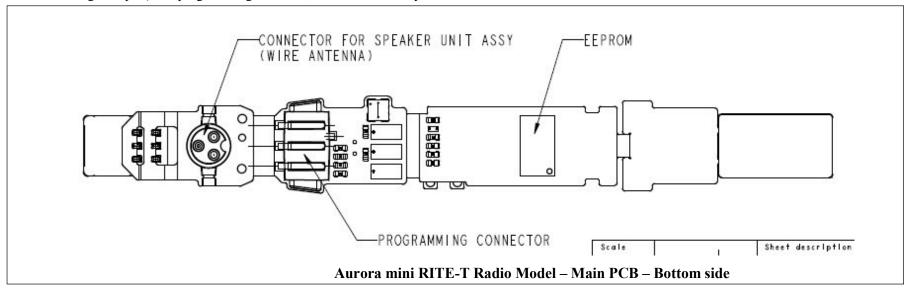
The most important parts inside the Engine module are a Digital-Signal-Processor (DSP), a radio Front-End (FE) chip for the 3.84 MHz radio part and an RF chip for the Bluetooth radio part – all mounted on a small rigid PCB again mounted on the main flex PCB. The Aurora mini RITE-T radio model also includes all voltage regulators and buffered data programming inputs on board. The DSP is the main processor controlling the functionality of both radios in the Aurora mini RITE-T radio model.
