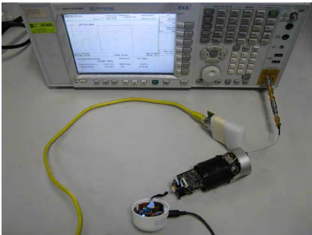
**CONDUCTED EMISSION SETUP**
