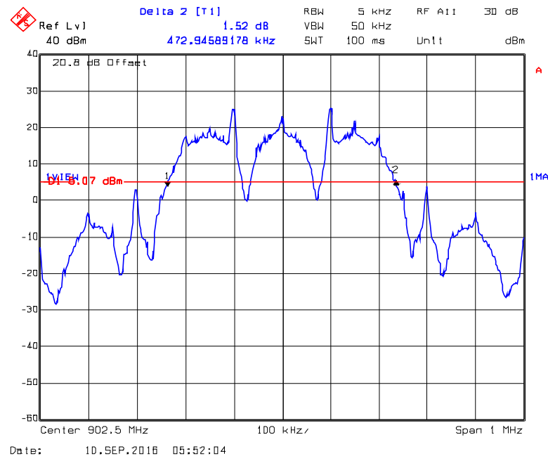
Plot 5.3.4.50. 20 dB Bandwidth, 902.5 MHz, DSSS4, 400 kbps- Right Antenna
