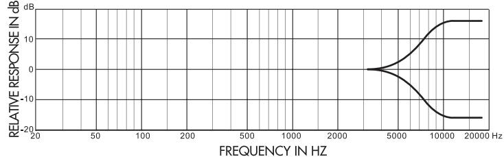
The high EQ control is a shelving EQ. What this means is that it boosts or cuts from 10kHz and everything above that. Turn it up to bring out the breath of a vocal or the high overtones of the cymbals. Turn it down to reduce finger squeaks on a guitar or bass.
